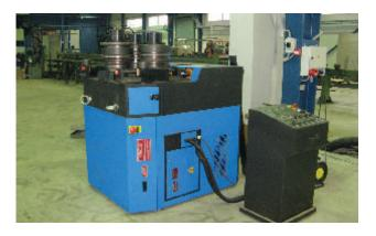
Profile Bending Machine with NC control Radius min 1 500 mm and blanks up to 160  $\times$  160 mm
