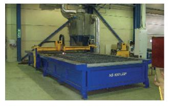
CNC Plasma Cutting Bench Cutting material up to 12 mm; working table 2 000  $\times$  6 000 mm
