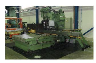
CNC Sheet Drilling Bench Material thickness up to 40 mm; working table 1 000  $\times$  2 000 mm; max hole 40 mm; 3 drilling heads
