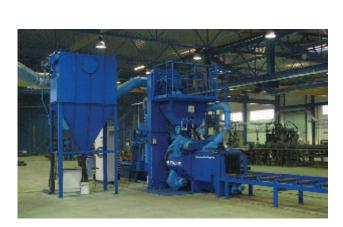
Shot Blasting Bench Details up to  $500 \times 520 \times 18~000~\text{mm}$
