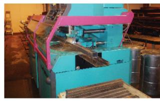
Circular Saw with NC control Detail diameter up to 120 mm; max detail length up to 11,7 m
