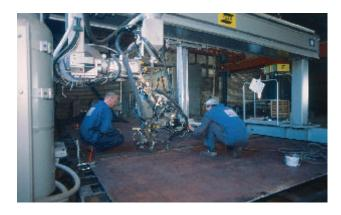
Submerged Arc Welding ESAB 1250A For the production of welded beams: width up to 4 000 mm; height up to 1 400 mm; length up to 33 000 mm
